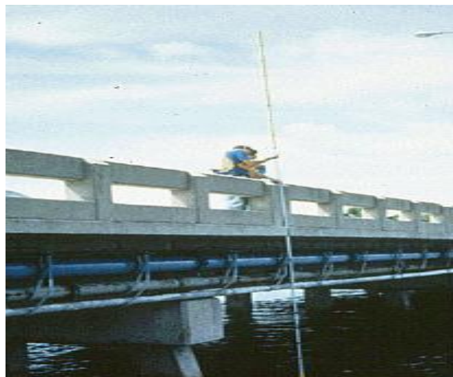
Figure 2-3 Sounding pole device (after Lagasse et al. 2001).
