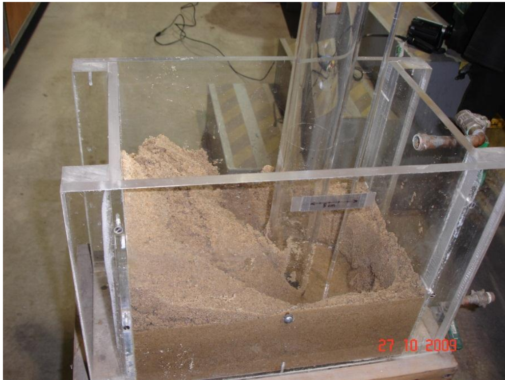
Figure 5-11 Leopold chain method experimental setup to quantify scour around a model bridge pier.
